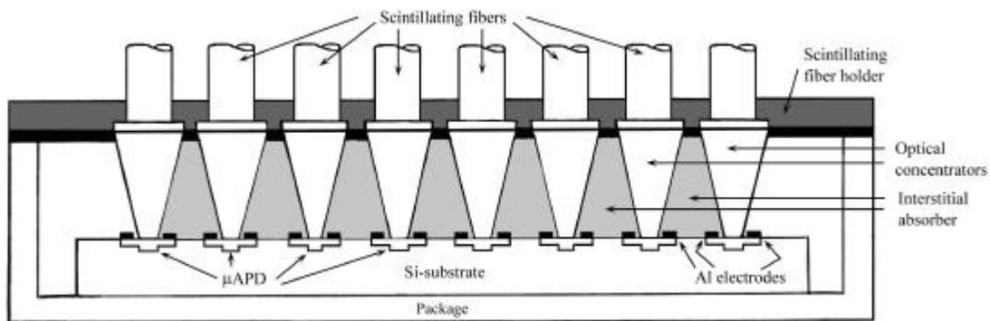
Figure 1. View of the envisaged integrated detector array. A coherent array of concentrators will be aligned and cemented to the sensitive area of the  $\mu$ APD pixels. Scintillating fibers are aligned to the concentrator arrays using a fiber connector. Quenching circuits may be mounted in the same package with the  $\mu$ APD array, thus resulting in a compact, multi-chip module.
