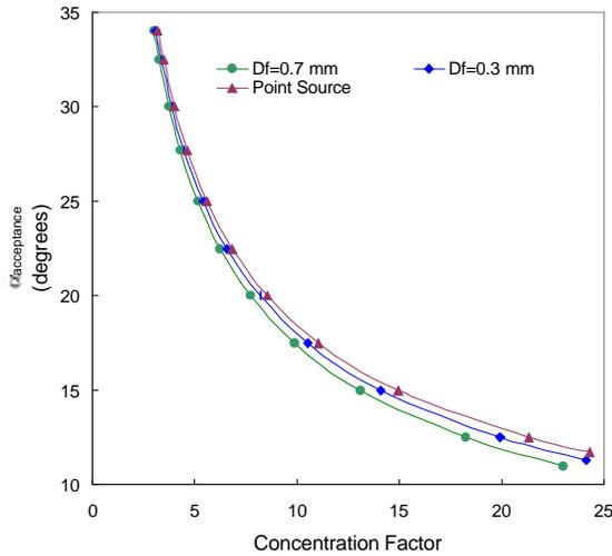
Figure 3. Calculated maximum acceptance angle versus the concentration factor for different fiber diameters. For high concentration factors, the acceptance angle will be smaller than the incident angle of the rays emitted by the scintillating fiber, and consequently light losses will occur due to back-reflection.
