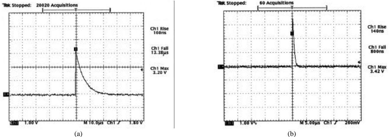
Figure 5 (a). Geiger pulse passively quenched using an active load quenching circuit with 20 k $\Omega$  resistors for 30  $\mu$ m diameter  $\mu$ APDs. The reset time is 14  $\mu$ s (horizontal scale is 10 $\mu$ sec/div); (b) Active load quenched pulse with 1 k $\Omega$  active load (horizontal scale is 5  $\mu$ sec/div). The reset time is 940 ns, and meets the FiberGLAST timing specification.
