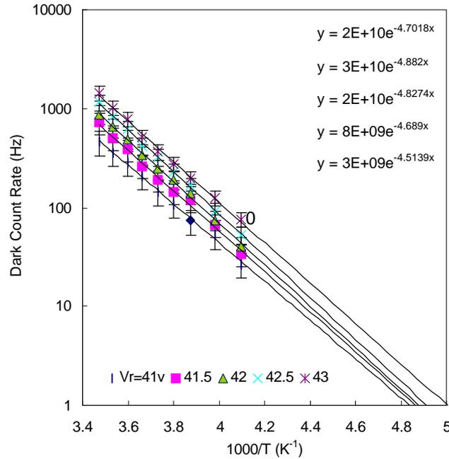
Figure 7. Measured and extrapolated dependence of the dark count rate on temperature for 30  $\mu\text{m}$  diameter  $\mu\text{APD}$ . Inserts show the fitted analytical functions associated with each applied voltage. These analytical functions will be used to predict the overall  $\mu\text{APD}$ -concentrator performance. The top inserted function corresponds to the highest applied voltage (43 V).
