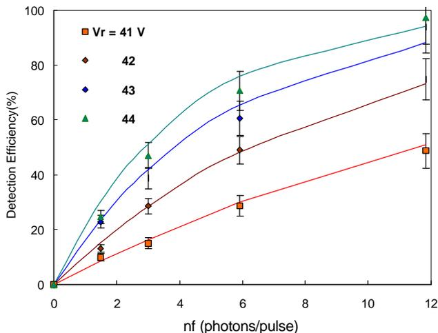
Figure 4. Room temperature measured  $\mu$ APD detection efficiency versus the number of photons,  $n_f$ , incident on the sensitive area. The experimental data are fitted with a saturation-type function.
