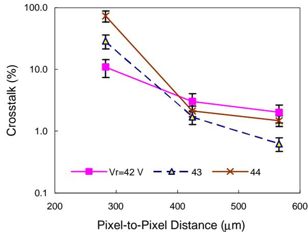
Figure 6. The dependence of the crosstalk on the distance between  $\mu$ APD pixels. The crosstalk was measured up to a voltage corresponding to the detection efficiency quasi-saturation condition. The crosstalk is less than 10% for pixel pitch greater than 380  $\mu\text{m}$  and decreases to approximately 2% for pitch sizes larger than 450  $\mu\text{m}$ .
